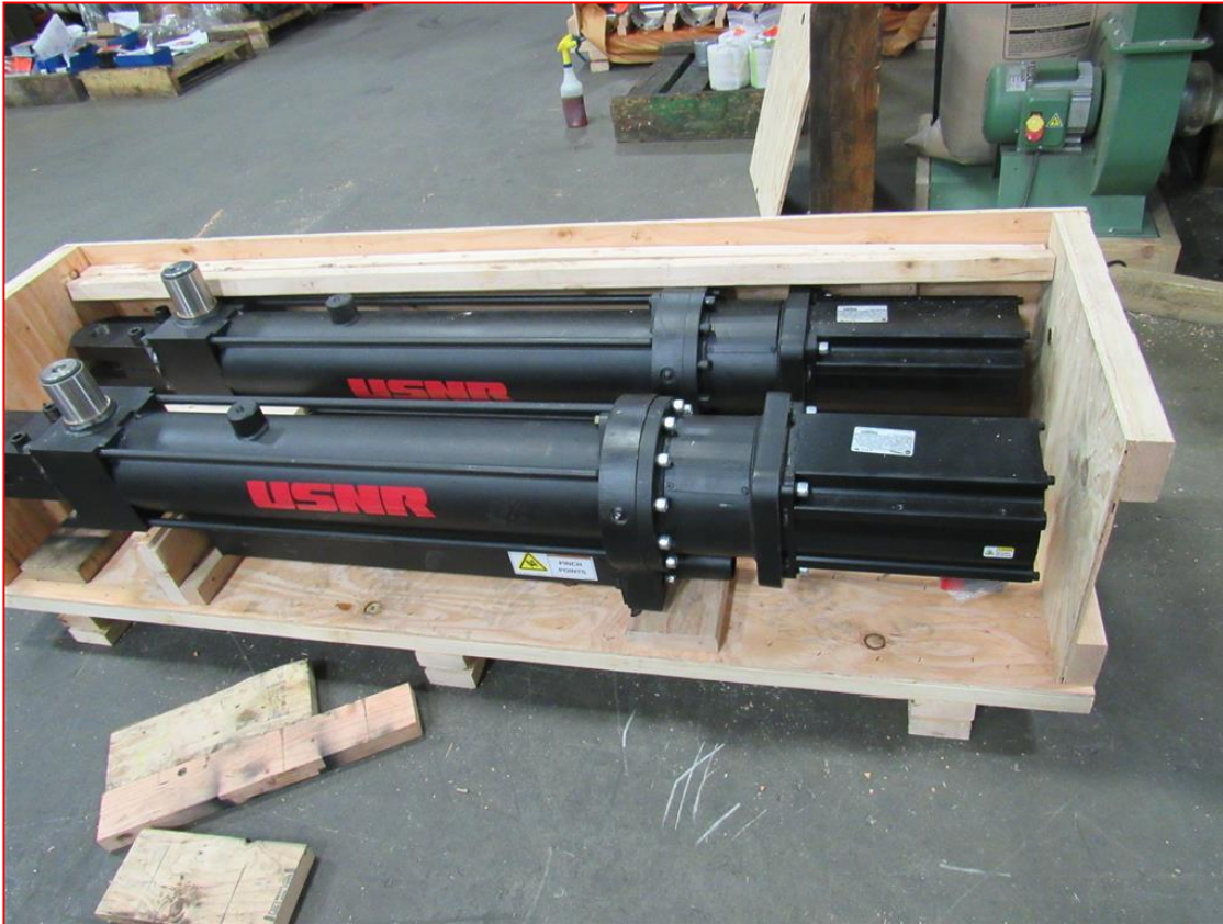
Assembled Actuators Approximately 700# Each
