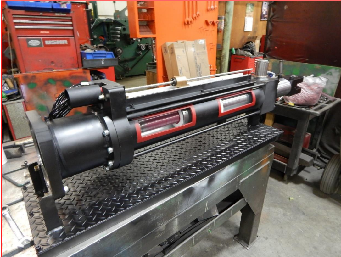
Actuator with Cut-a-way Showing Screw Assembly
