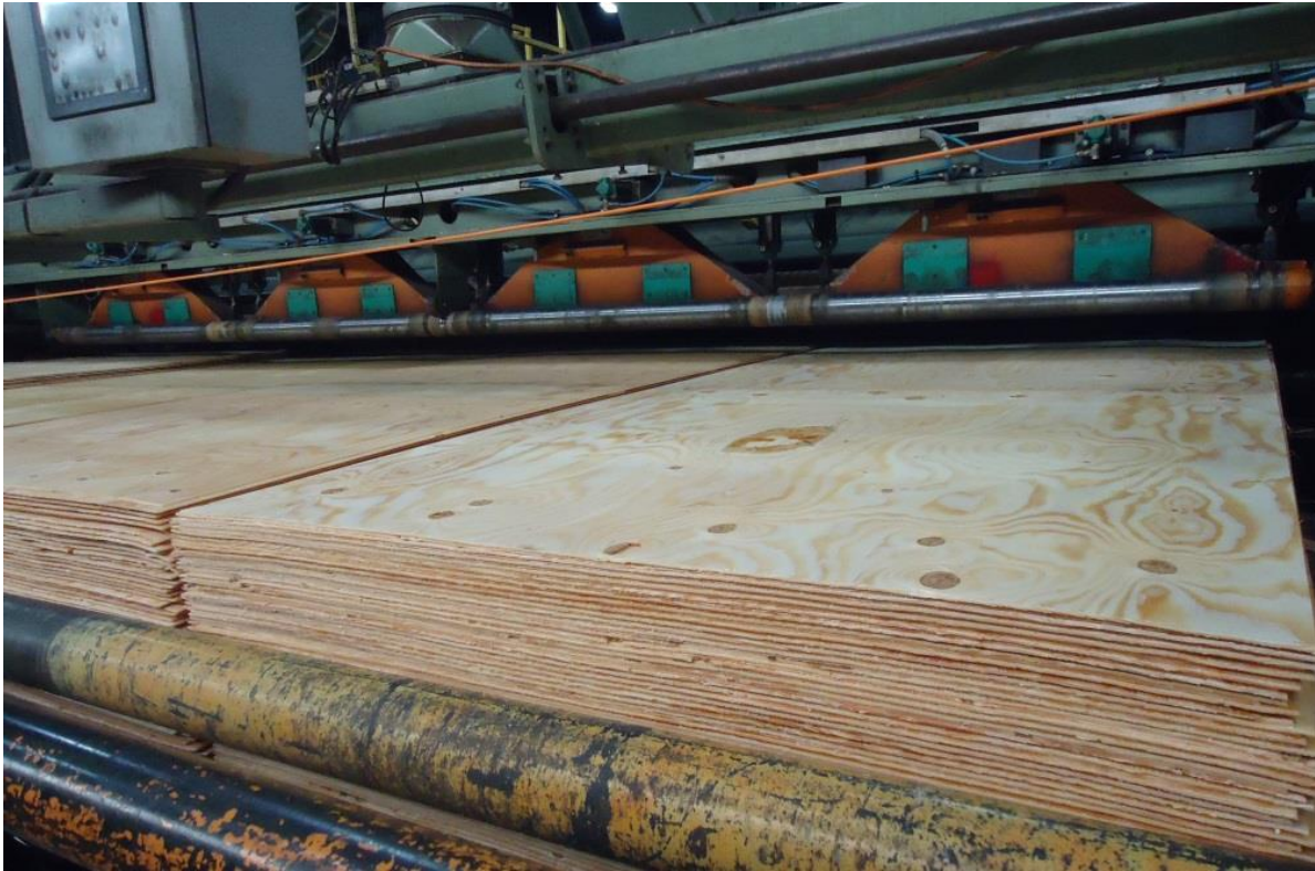
Very flat stacked veneer, sound knots
