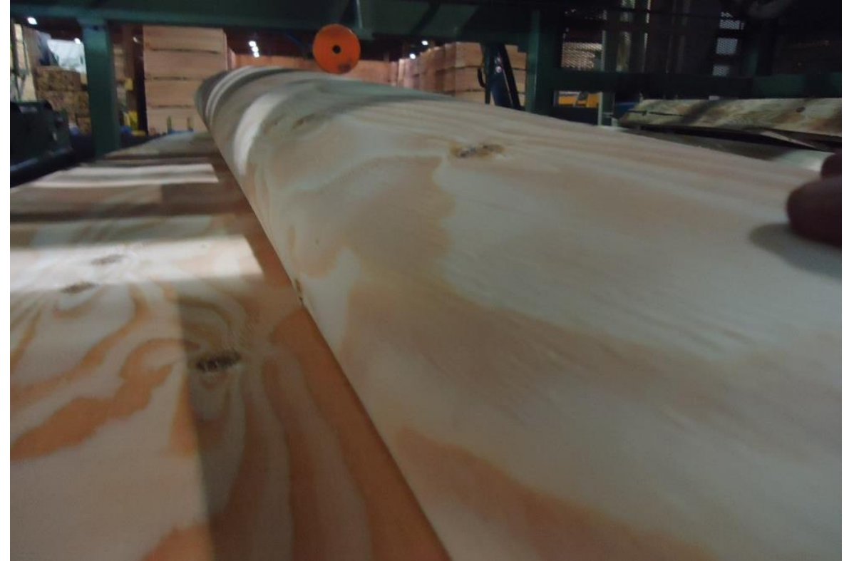
Very smooth surface with small lathe checks
