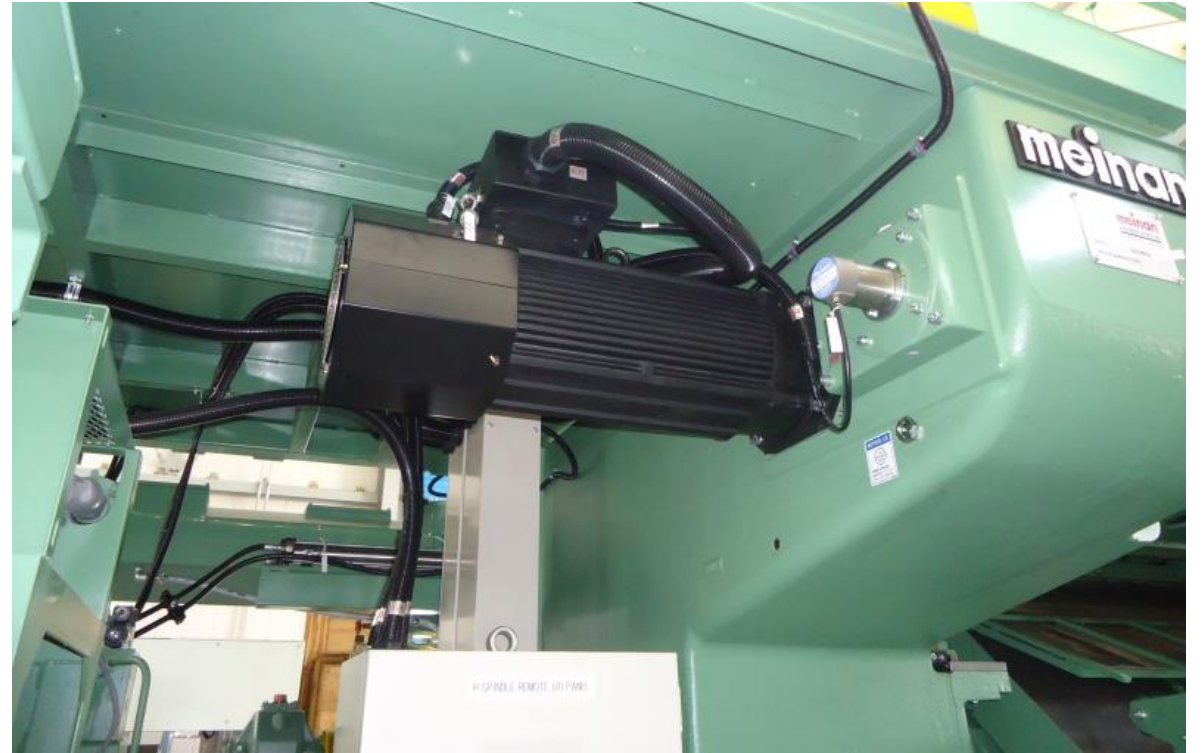
Single 30 HP AC servo motor – knife carriage
